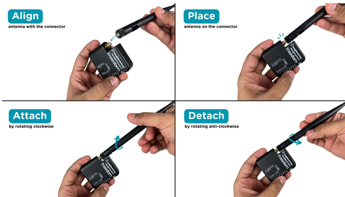
Fig. 2.2: Attaching antenna to BeagleConnect Freedom
